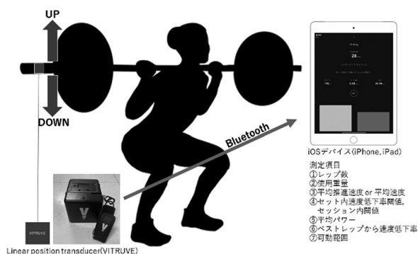
Fig. 2. Strength training using a linear encoder (VTRUVE®, Spain)
